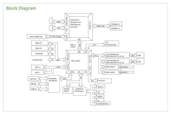
2 x ports by 2 x 5-pins header pitch 2.54mm (port 4  $\sim$  5) 2 x ports to Mini-PCle slots (port 6, 7)
