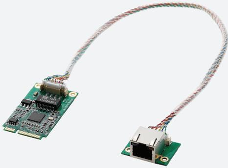
**NISKLAN03 without bracket, cable length 250mm
