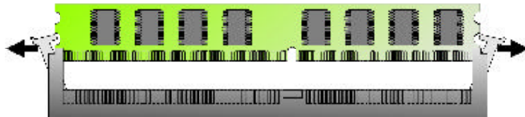
Figure 3-4 : How to Install DIMM (4)
